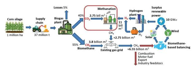
Figure 7. Concept of conversion of green hydrogen to synthetic methane
